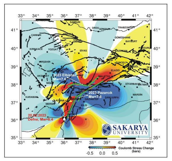
**Figure 6.** Coulomb stress changes due to the 2023 Pazarcık and Elbistan eartquakes calculated along the fault plane of the February 20, 2023 Defne aftershock.
