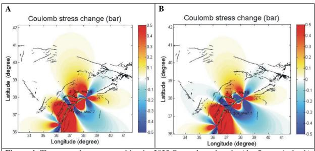
**Figure 4.** The stress changes caused by the 2023 Pazarcık earthquake (the first mainshock) calculated (**a**) along a fault with parameters  $285^{\circ}$ , dip  $90^{\circ}$  and rake  $0^{\circ}$ , representing the fault segment that host the 2023 Elbistan earthquake's (the second mainshock) epicenter, and (**b**) along a fault with parameters  $274^{\circ}$ , dip  $90^{\circ}$  and rake  $0^{\circ}$ . After Utkucu et al. (2023b).
